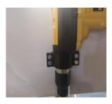
Slide the drill back into the clamp until it touches the casing
