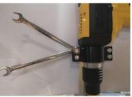
Tighten the 4x M8 nuts/bolts until the drill is secure
